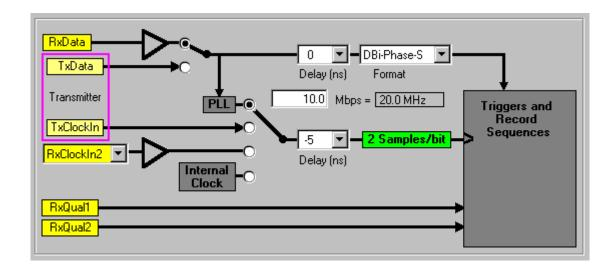
The input format defines the encoding (e.g. NRZ-L) that is expected on the receive data. This choice has an affect on many other elements of the receive channel including clock rate, number of clocks per bit, trigger patterns and trigger count. See the following Data Formats section for more information on data encoding issues.
