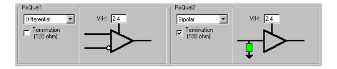
The threshold voltage range is dependent on the receiver front-end module. The voltage ranges for the front-end modules are shown below.
