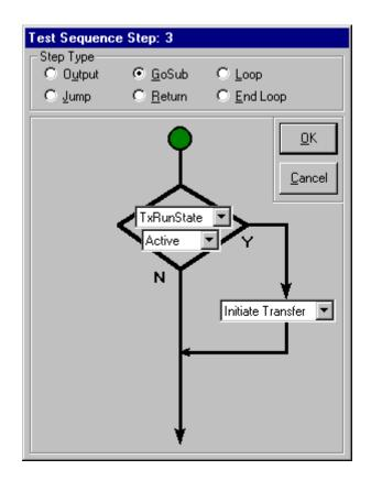
The RxTrigger condition provides a way to dynamically respond to a receive trigger that occurs. When the RxTrigger condition is set to True, the destination drop-down list includes an entry for a subroutine vector table (i.e. <Subroutine Table>). This refers to the RxTrigger Subroutine Table that associates subroutines with triggers defined in a Record Sequence window. Thus, the executed subroutine is dependent on the trigger that causes RxTrigger to be True.
