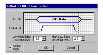
The Active High checkbox controls the polarity of the offset signal display. This allows the offsets to be shown according to the programmed, or selected polarity, of the physical signal. TxMarker levels are individually defined within a Control Memory Table window. Output signal polarity is controlled in the Signal Pinout window.
