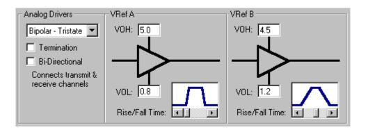
The output voltage ranges are dependent on the transmitter front-end module. In all cases the high output voltage must be greater than the low output voltage (i.e. VOH > VOL). The voltage ranges for the front-end modules are shown below.
