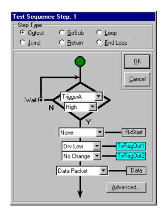
The RxStart drop-down list identifies a record sequence step to activate. Record sequences are armed for a single step or a series of steps. The levels of TxFlagOut1 and TxFlagOut2 may be set to high or low, or left unchanged, during an Output test sequence step.
