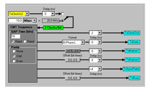
The output format defines the encoding (e.g. NRZ-L) that is applied to TxData before it is transmitted. This choice has an affect on many other elements of the transmit channel including clock rate, number of clocks per bit, offset timing and Waveform Parameter Registers. See the following Data Formats section for more information on transmitter encoding.
