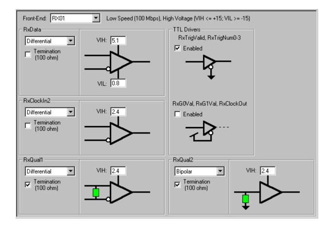
Termination can be added on the input signals by a left mouse click on the appropriate Termination checkbox. Input termination is a parallel impedance of 100 ohms. If the TTL output signals are not needed, they can be disabled to minimize signal noise.
